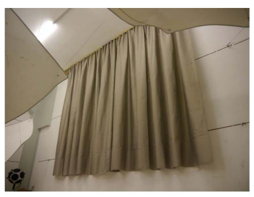
Figure B.4. Folded arrangement, test arrangement in the reverberation room: diagonal view.
