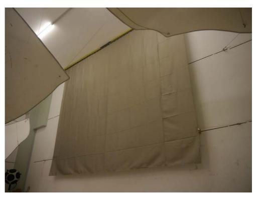
Figure B.2. Flat arrangement, test arrangement in the reverberation room: diagonal view.
